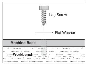
Figure 9. Example of a direct mount setup.
